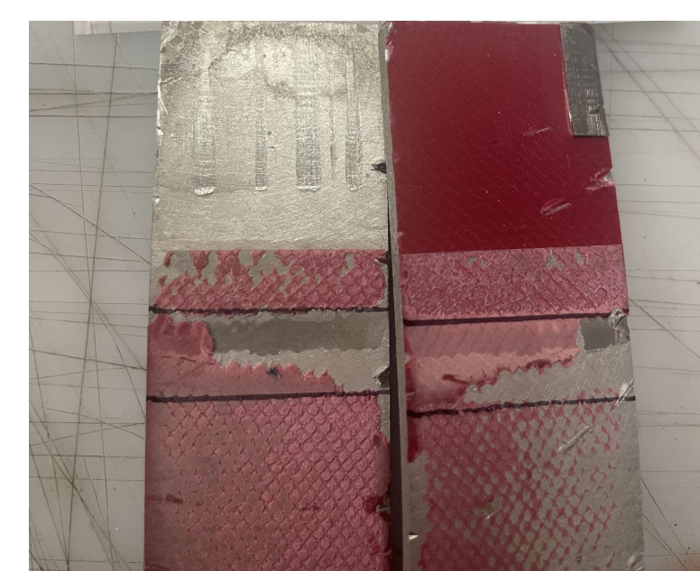
Fig. 3: 1-layer wedge crack test sample 1
